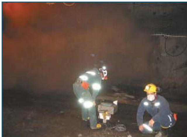
was tested side-by-side with the millimetre-wave sensor. To simulate an opaque dust cloud, a bag of cement and ore dust was dispersed in a mine tunnel using compressed air and powerful fans as shown in Figure 2.
