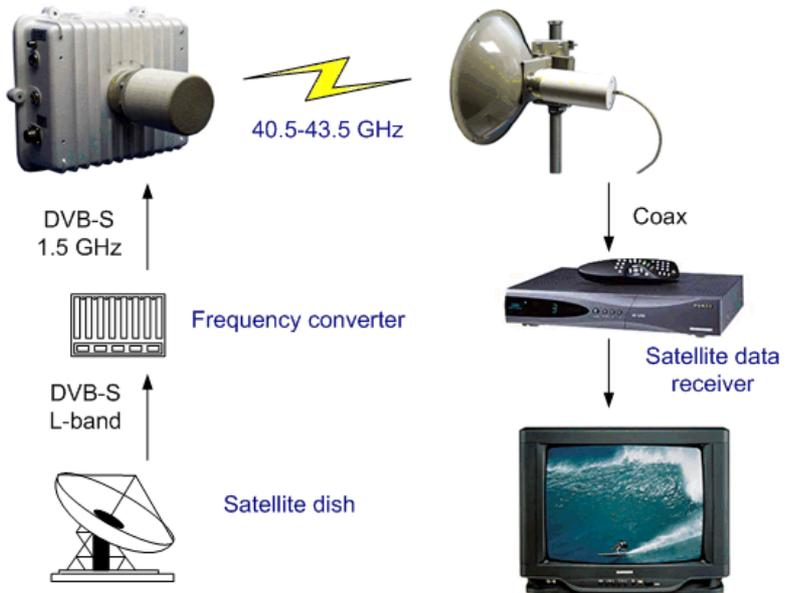
To broadcast DVB-ASI/SPI stream, DVB-S modulator should be used.
